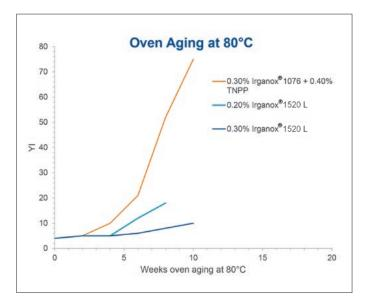
Improved color stability of high cis BR during oven aging at  $80^{\circ}\text{C}$  with Irganox® 1520 L
