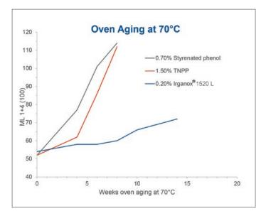
Stable Mooney viscosity after oven aging at 70 °C of E-SBR with significantly lower amount of Irganox® 1520 L compared to classical phenolic or phosphite antioxidants for E-SBR
