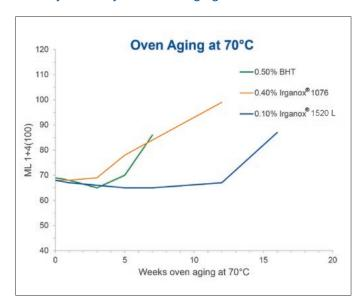
Longer thermal stability of S-SBR at 70°C with much lower concentration of Irganox® 1520 L compared to standard phenolic antioxidants
