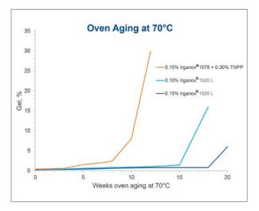
Significant reduction in gel formation in low cis BR during oven aging at 70°C with much lower antioxidant concentration
